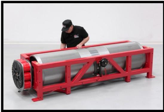
Super-duty dynamometer frame assembly – mating this 30” “traction grooved” high-inertia roller, together with Land & Sea’s large-diameter direct-drive eddy absorber.
