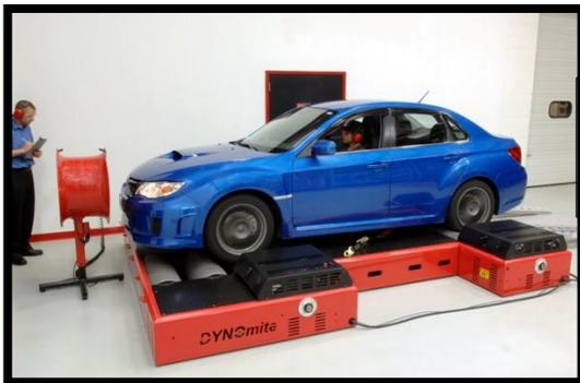
Our “multi-roll” mechanically-linked AWD dynamometer option allows hassle-free testing of FWD or RWD traction-controlled vehicles, as well as 4WD and AWD applications.
