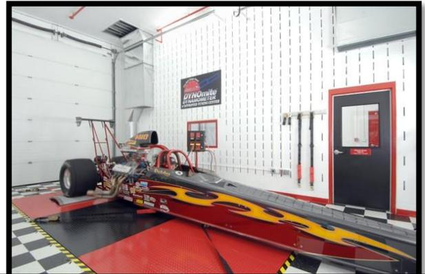
One of Land & Sea's own AWD bays uses adjustable I-beams, supporting over-sized pit plates, to accommodate our testing of numerous configurations of production chassis dynamometers.
