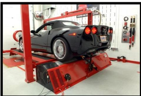
20-inch roll system is available with eddy-current absorber and/or AC motoring options. Installs in a pit or above ground – with optional four-post lift (as shown) or ramps.
