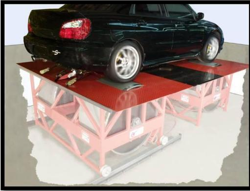
Adjustable wheelbase in-ground 44-inch AWD twin-roll dynos (with or without absorbers) handle 3,000+ Hp at 225 MPH. Mechanical (or optional electronic) roll synchronization.
