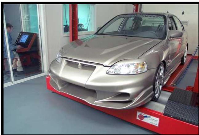
DYNOmite 13-inch tandem quad-roll assembly with absorber, loads to 150+ MPH and 700+ wheel Hp (AWD optional). Mounts in the ground or above (ramps included).
