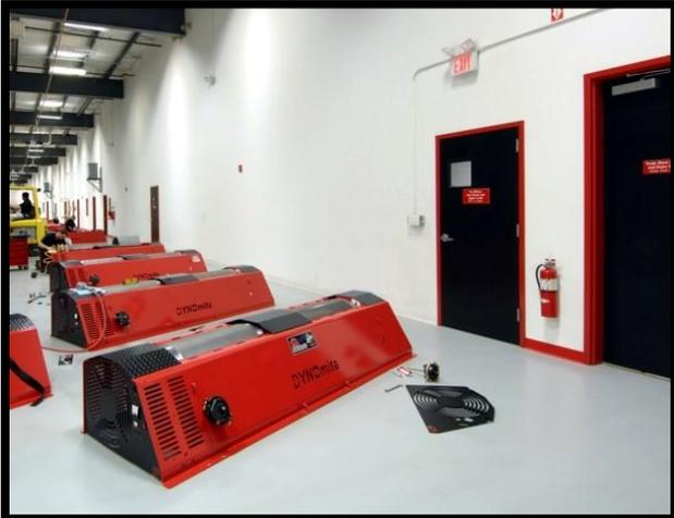
FWD/RWD or AWD (to 1,500+ Hp\*) chassis kits include: 8½", 13", or 20" medium-inertia dual-roller assembly, removable roller shield, drive-up ramps, wheel chocks, casters, water or eddy-current absorber with step-up drive, electronic torque transducer, DYNOmite data-acquisition computer, AC power supply, electronic auto-load control, DYNO-MAX software, inductive RPM pickup, required hoses, engine-temperature thermistor, and full-function data harness.
