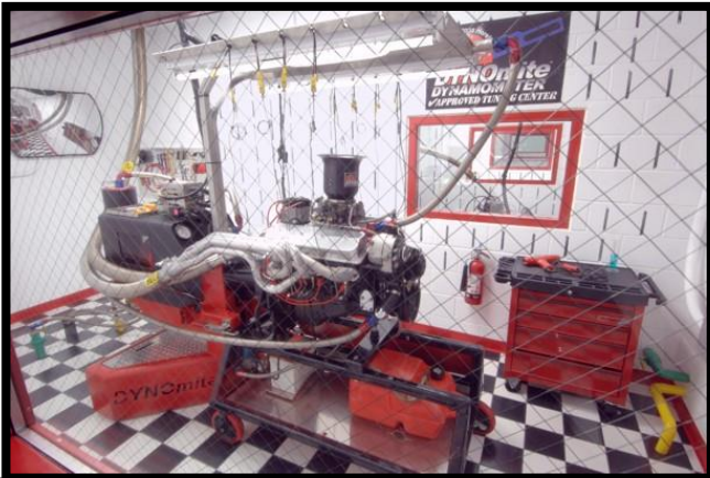
Here is a look, through the sound-proof safety glass, into one of Land & Sea's several engine dynamometer test and training cells.
