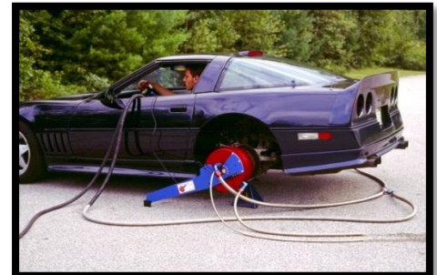
DYNOmite rear-wheel brake on 1988 Callaway Turbo Corvette. Only Land & Sea, Inc. has a long history of offering AC, eddy-current, hydraulic, and even hybrid-absorber axle-hub dynamometer solutions.
