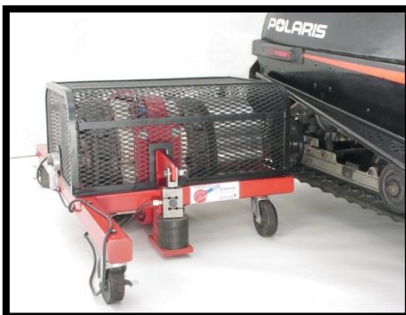
DYNOmite eddy-current track (or clutch only) driven dynos. Custom designed for snowmobile OEM's load simulation and Hp.
