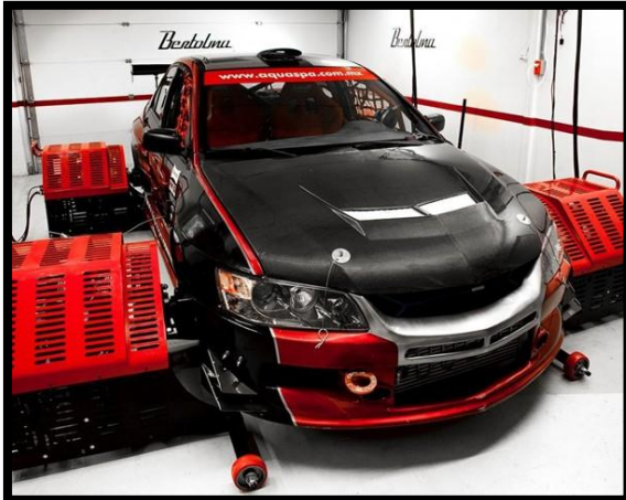
DYNOmite AWD axle-hub dynamometers, on EVO 9, at Bertolina's dyno facility.
