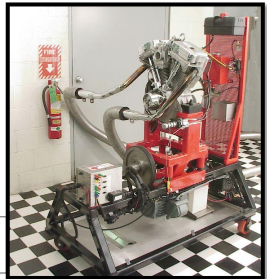
Custom DYNOmite V-twin motorcycle engine dynamometers... that were developed for this manufacturer's end-of-line production testing.
