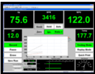
Custom DYNOmite V-twin motorcycle engine dynamometers... that were developed for this manufacturer's end-of-line production testing.
