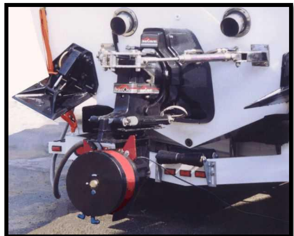
800 Hp dual-stator absorber (with Siamese rotor) tests high-power blower engines... without costly engine removal.
