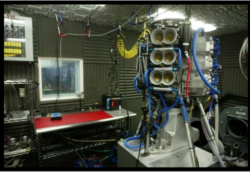
400 Marine Engine Dyno Kit – makes dry-land testing conclusive. Bidirectional absorber tests either CW or CCW-rotation engines. (Shown without carrying case.)
