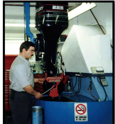
Engine cooling can be provided with a small test tank, your yard’s flushing supply, or even direct submersion at the boat
